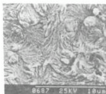
Fig.1 Morphology of unstretched specimen by SEM
